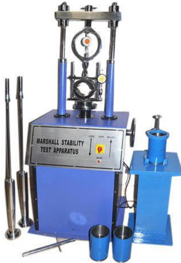
FIG.3.7. MARSHALL STABILITY TESTING MACHINE
