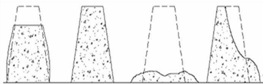
True Slump Zero Slump Collapsed Slump Shear Slump potentially non-plastic potentially non-cohesive no displaced center
