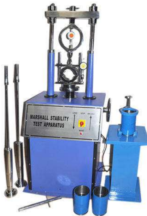
FIG.3.7. MARSHALL STABILITY TESTING MACHINE
