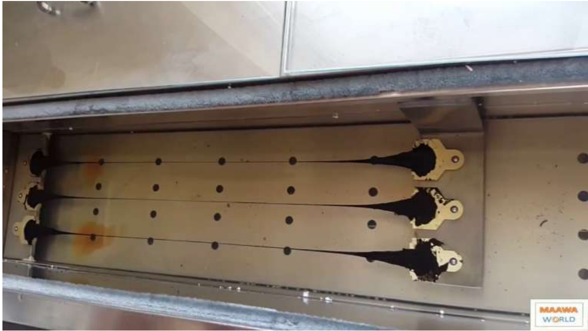
FIG.3.3 CONCEPT OF DUCTILITY TEST
